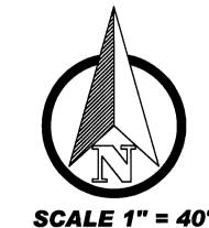
BEARINGS are based upon Indiana West State Plane Coordinates (NAD83), established by RTK GPS observations using INDOT VRS network
