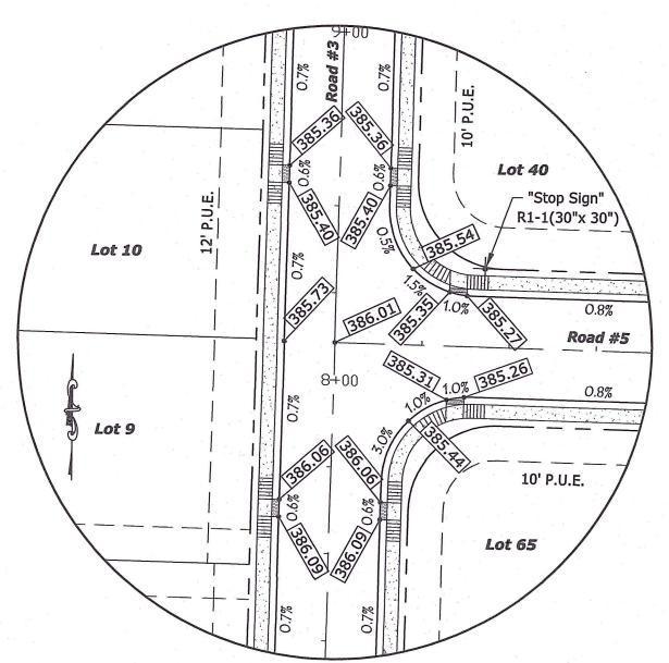
Note: All elevations along curb line are gutter elevations. Raise 0.33' for top of curb elevation.
