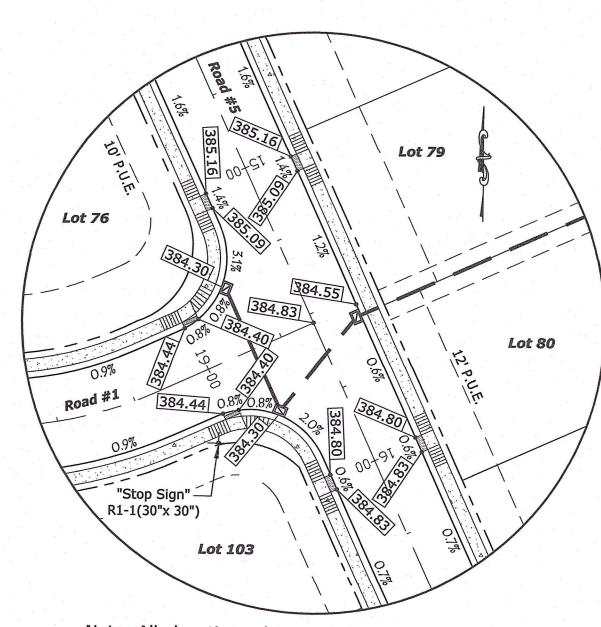
Note: All elevations along curb line are gutter elevations. Raise 0.33' for top of curb elevation.
