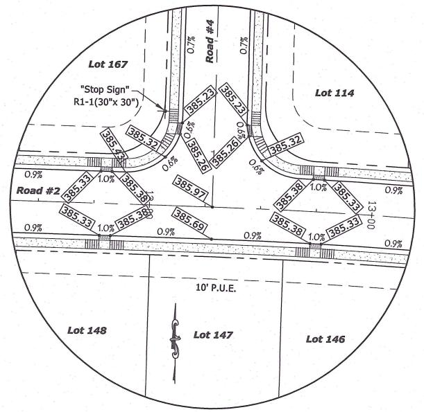
Note: All elevations along curb line are gutter elevations. Raise 0.33' for top of curb elevation.
