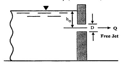
P131 **Outflow Pipe** Flow Characteristics 18 Pipe Dia. (inch) Orifice diameter 16.00 D (inch) A<sub>o</sub> (s.f.) Area of orifice 1.40  $g(f/s^2)$ Acceleration due to gravity 32.2 Head at Inlet H (ft) 4.50 Head at center of orifice h<sub>o</sub> (ft) 3.83 Discharge coefficient for sharp edged orifice plate  $C_d$ 0.61
