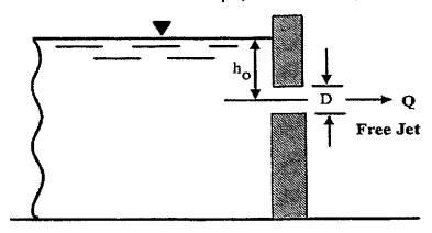
P101 **Outflow Pipe** Flow Characteristics 12 Pipe Dia. (inch) Orifice diameter 11.00 D (inch) Area of orifice  $A_o$  (s.f.) 0.66 Acceleration due to gravity  $g(f/s^2)$ 32.2 Head at Inlet H (ft) 4.00 Head at center of orifice h<sub>o</sub> (ft) 3.54 Discharge coefficient for sharp edged orifice plate 0.61  $C^q$
