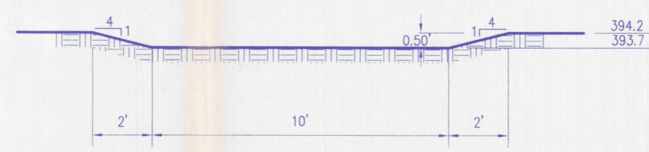
Retention Basin Emergency Spillway No Scale
